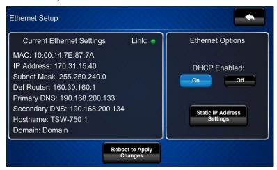
The "Ethernet Setup" menu displays the touch screen's *Mac* and *IP Address*, *Subnet Mask*, *Def Router*, *Primary DNS*, *Secondary DNS*, *Hostname* and *Domain*. There are controls for turning *DHCP* **On** or **Off** as well as a **Static IP Settings** button, which provides access to controls which allow editing of these settings. This screen also contains a *Link* indicator to show the status of the Ethernet connection.
