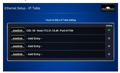
The "Ethernet Setup – IP Table" menu displays up to four IP table settings, each of which has an *Online* indicator. To add or edit an entry, touch the **Add/Edit** button to its left. The "Ethernet Setup – Edit IP Table Entry" screen is displayed.
