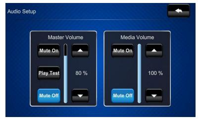
The "Audio Setup" screen provides controls for muting (or unmuting) the audio, adjusting level for both *Master Volume* and *Media Volume*, as well as a control for
