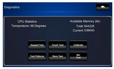
The "Diagnostics" menu displays the CPU temperature, *Available Memory* and contains controls to run a **Keypad Test**, **Touch Test**, **Rava Test** and **Mic Test**. In addition there are controls to initiate touch screen calibration and to open various test screens. These are explained in the paragraphs that follow.
