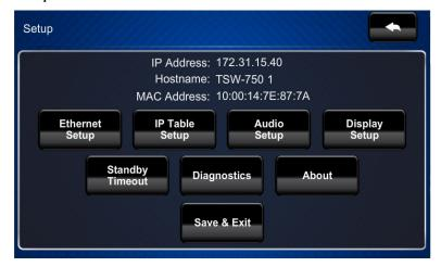
The "Setup" menu is comprised of buttons for Ethernet Setup, IP Table Setup, Audio Setup, Display Setup, Standby Timeout and Diagnostics. In addition, there is an About button that provides information about the touch screen and a Save & Exit button. The functions of each are detailed in the next section of this guide.
