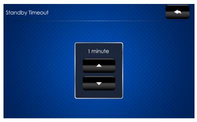
The "Standby Timeout" screen provides controls to adjust standby timeout from 0 to 120 minutes.
