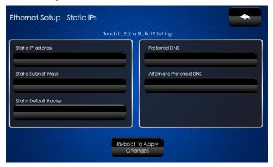
To edit the *Static IP Address*, *Static Subnet Mask*, *Static Default Router*, *Preferred DNS* or *Alternate Preferred DNS*, touch the button directly under the label for the entry to edit. The on-screen numeric keypad opens.
