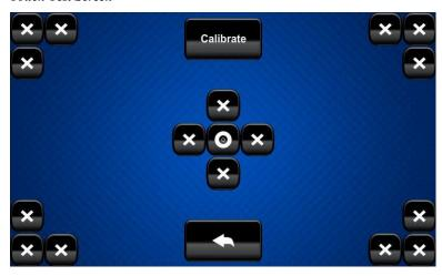
The touch test screen can be used to test the function of the screen. When a location button (the "x" buttons or the "o" button) is touched, its indication on the screen lights. This screen also contains a **Calibrate** button to initiate touch screen calibration.
