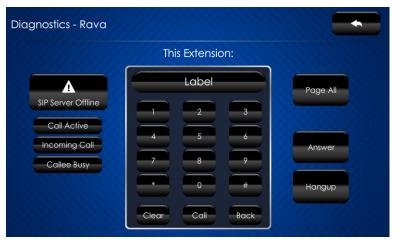
The "Diagnostics - Rava" screen provides controls for testing the use of Crestron's Rava<sup>TM</sup> SIP Intercom with the TSW-550/750/1050. They can be used to test projects and settings. If the intercom works but the project does not, there is an issue with the project; if the intercom does not work, there is an issue with the settings.
