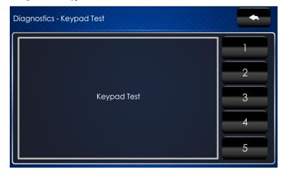
The "Diagnostics - Keypad" screen can be used to test the function of the hard key push buttons on the right side of the screen. When a button is pressed, its corresponding indication on the screen lights.
