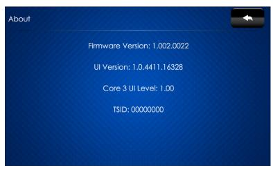
The "About" screen displays information about the touch screen, including the currently loaded firmware and operating system versions.
